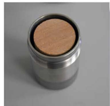
Sample holder with core specimen
