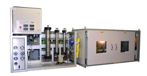
They are then expanded to atmospheric pressure and temperature through a back pressure regulator. An ultrasonic multiphase separator for liquid measurement as the produced gas is measured by a wet gas meter.
