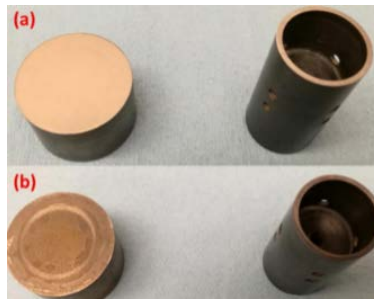
Figure 4 - a) DLT steel and rubbing shoe, b) Steel block after test with a visible “ring”
