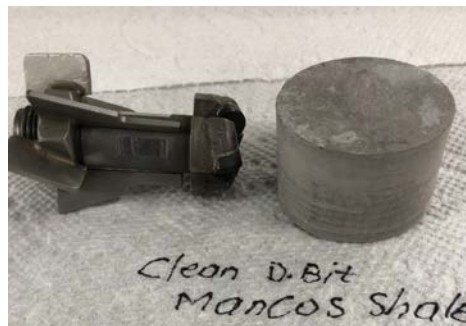
Figure 11 – DS accessories. Drill bit with spindle blade (left). Mancos core drilled to 7/8 inch with total 1.5inch diameter and 1inch height (right).
